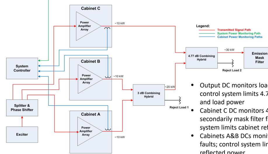
Output DC monitors load reflected power; control system limits 4.77 dB hybrid, filter,
