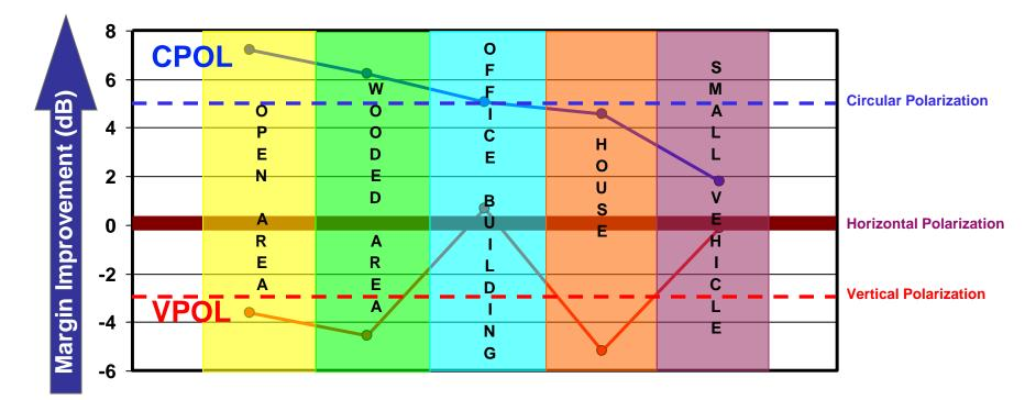
On average, circular polarization offers 5 dB margin improvement over horizontal polarization
