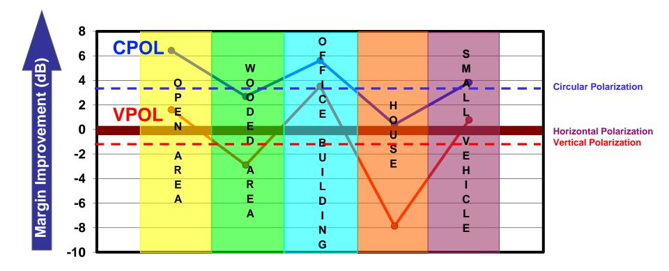
On average, circular polarization offers 3.5 dB margin improvement over horizontal polarization
