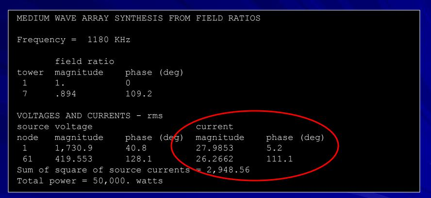
Normalize phase (111.1 – 5.2), Tower 7 Phase =  $+105.9^{\circ}$ Ratio current (26.2662 / 27.9853), Tower 7 Ratio = 0.939
