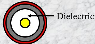
Velocity of Propagation = Vp Polyethylene = 66%Teflon = 70%Foam = 78%, 84%, 86%
