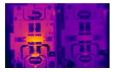
Temperatures of Doherty Amplifier transistors compared to standard Fixed Drain Class A/B
