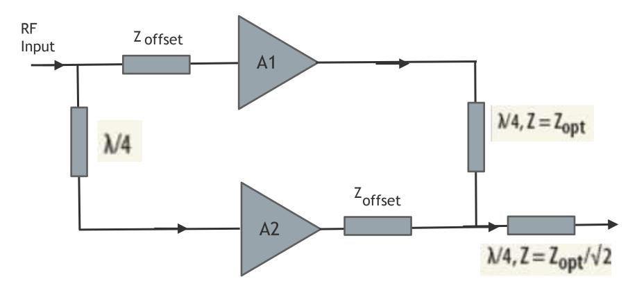
A basic **DOHERTY** architecture contains a carrier amplifier biased to operate in Class AB mode (A2) and a peaking amplifier biased to operate in Class C mode (A1).
