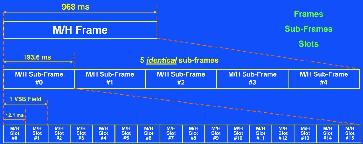
1 M/H Frame = 5 M/H Sub-Frames = 80 M/H Slots = 40 8-VSB Data Fields Adding M/H technology does *NOT* change VSB data frame structure
