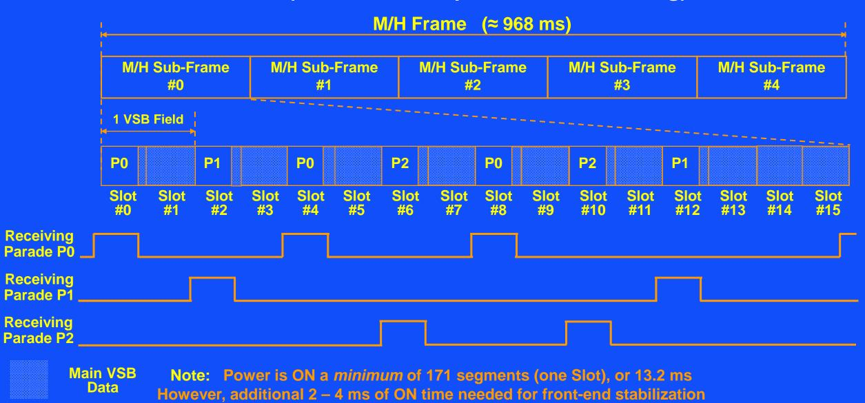
**Burst transmission allows battery conservation**
