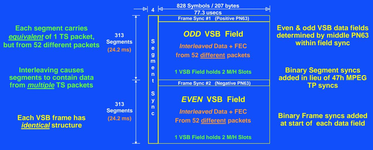
VSB symbol domain <u>after</u> convolutional data byte interleaving
