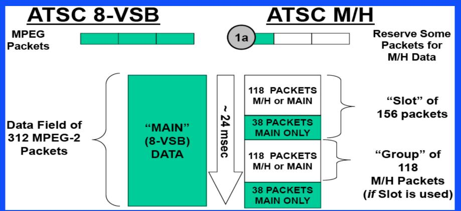
Each Slot has a section for Main packets & one for M/H packets Each Slot may <u>or</u> may not contain M/H data Each Slot carries 156 data packets (156 Main <u>or</u> 118 M/H + 38 Main) 2 M/H Slots transmitted per 8-VSB Data Field M/H Frame *offset* from VSB field Sync by 37 packets
