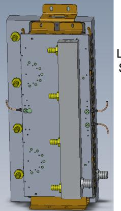
Liquid cooled 14-Way Splitter & ISO-Loads
