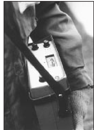
Figure 3. ComSonics leakage-detection meter. For simplicity, the meter is calibrated in red, yellow, and green bands rather than microvolts per meter. Red indicates an excessive egress level.
