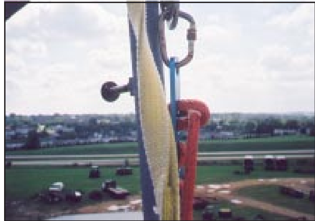
Figure 3. Lanyard, carabiner, rope terminator, and kern mantle rope.
