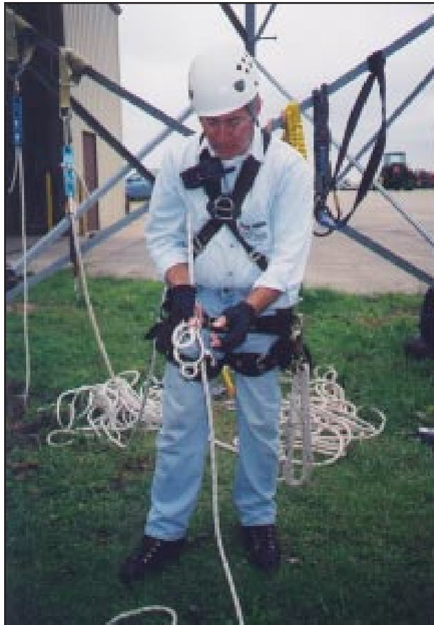
Figure 4. Ed Van Ness demonstrates how to properly insert kern mantle rope through a Fisk descender.
