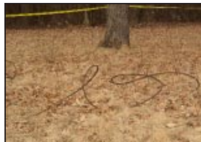
Figure 9. Untensioned guy wire curls into spirals.
