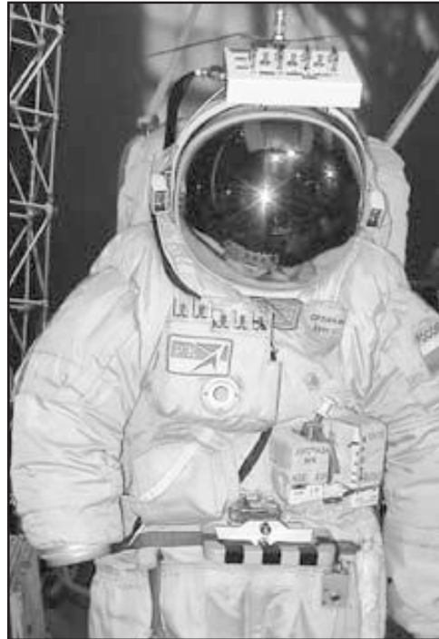
Figure 1. SuitSat in its flight configuration. The electronics control panel is on the top of the helmet along with the SuitSat antenna. [Photo courtesy of Energia, from the AMSAT.org web site]
