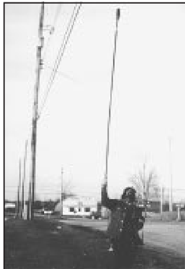
Figure 2. Measuring egress with ComSonics leakage-detection equipment, Flint, Michigan, 1982. The pickup antenna is a helical coil inside a plastic housing, an arrangement accepted by the FCC based on tests provided by the antenna manufacturer.
