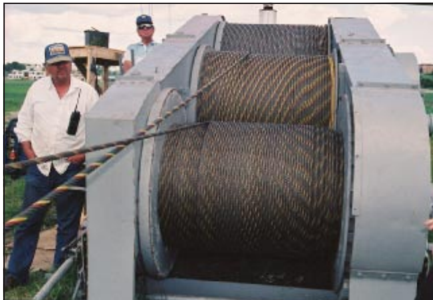
Figure 1. Three-drum winch used for Madison Candelabra DTV project.
