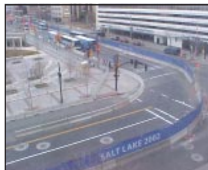
Figure 2. Security fences surrounding the Salt Palace Convention Center, photographed from the 12th floor of the Shilo Inn. The inside fence is located on the sidewalk; the outside fence runs down the center of the street.
