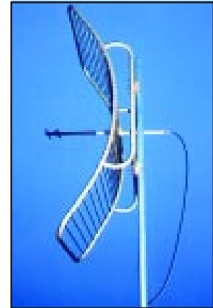
Figure 2. STL transmit antenna.
