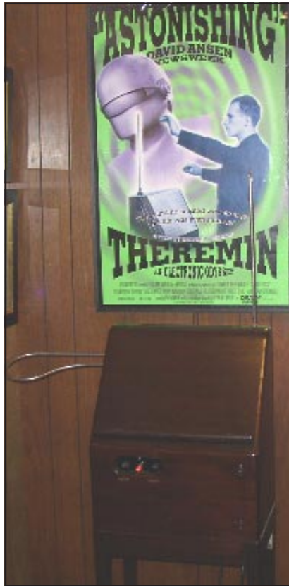
Figure 7. Theremin is played by moving hands near the antennas without touching them.
